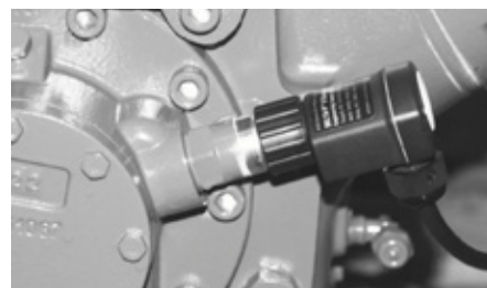
Oil pump with INT250 Switch pressure switch
